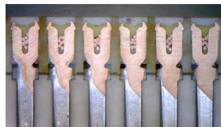
Step 9 - Place the sample under the microscope for etching and picture taking
